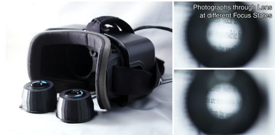
Figure 3. Photograph of HMD prototype and focus-tunable lens.
